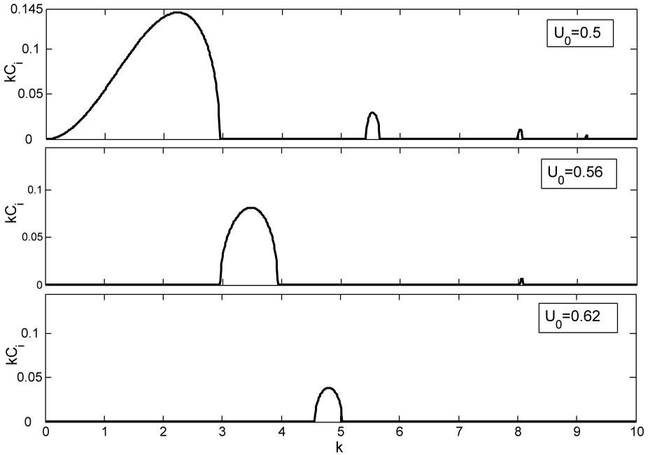
Figure 2. Instability curves,  $kC_i(k)$ , of the coupled density front ( $U_0 = 1/2$ , upper panel) and the coastal current ( $U_0 > 1/2$ , middle and lower panels) on the  $f$ -plane ( $\epsilon = 0$ ). The similarity between the two instabilities is evident despite the different  $V$ -boundary condition (but not that of  $\psi$ ) employed in the two problems. These instabilities vanish for  $U_0 \geq 0.65$ .
